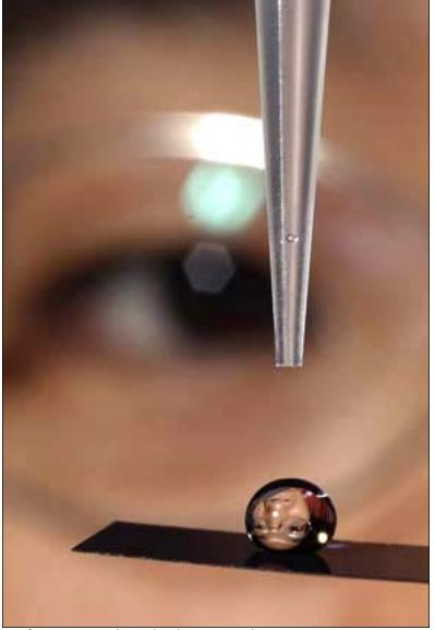
**Neal C. Lauron**, *The Columbus Dispatch* - 1st Portrait Nanofiber researcher Nan-Rong Chiou puts a drop of water on a piece of acetate coated with a polymer that is hydrophobic - not capable of uniting with or absorbing water.
